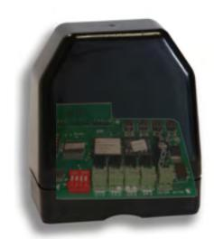
The outdoor use 4-channel DUCATI rolling coded adio receiver allows you to control up to 4 automatic devices of any type by means of any ducati rolling coded remote controls.
