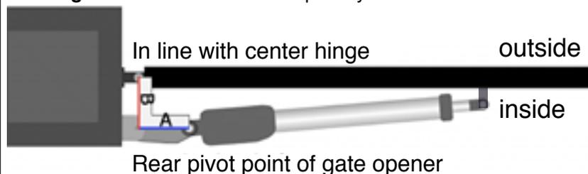
■ **A=** this measure must allow the actuator can open the gate wing at 90 °.
