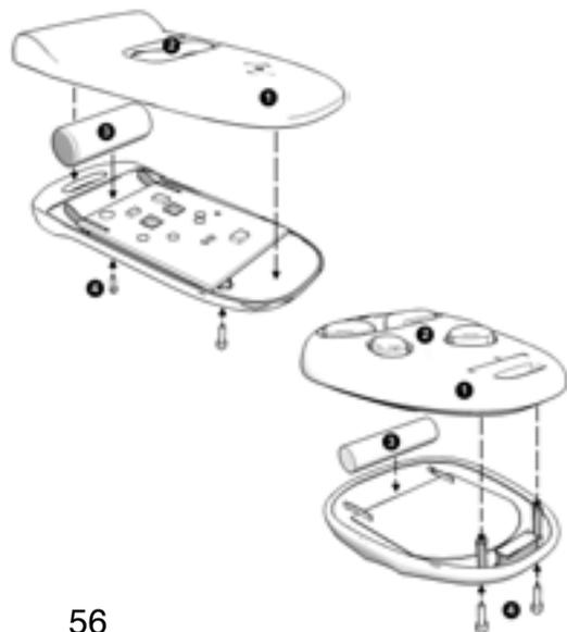
The DUCATI radio rolling coded transmitters (FOB), featuring a unique “rolling code” radio protocol are compatible with all Ducati rolling coded openers (CTH electronic boards). With over 3 billions of continuously changing combinations, they ensure maximum protection against radio interferences. Frequency: 433,92MHz
