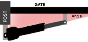
To ensure a perfect lock of the gate when closed, the actuator must be installed in way to have an angle of incidence to the gate wing in closed position.a greater angle ensures greater tightness
