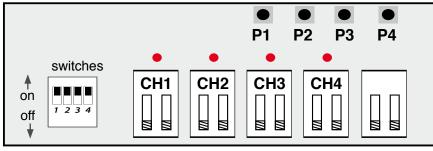
ON position = bistable contact: OFF position = monostable contact
