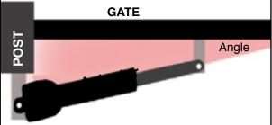
To ensure a perfect lock of the gate when closed, the actuator must be installed in way to have an angle of incidence to the gate wing in closed position.a greater angle ensures greater tightness
