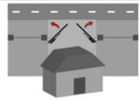
PUSH TO OPEN OPERATION (opens towards inside) If your driveway slopes up after the gate, preventing it from swinging in. This means the gate operator is mounted on the inside of the property and pushes your gate out away from the property. Warning:remember to reverse the polarity of the motor cables when connecting to the electronic board
