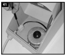
WARNING! To prevent damage during shipment, the transformer could be provided not pre-installed in the control panel. it is supplied with a fixing cone and screw to fix it to the bottom of the the control box.
